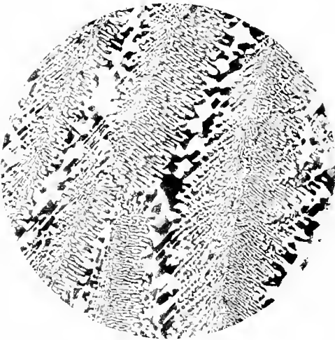
B. Eutectic alloy of antimony and \text{Cu}_2\text{Sb} . \times 200 .
